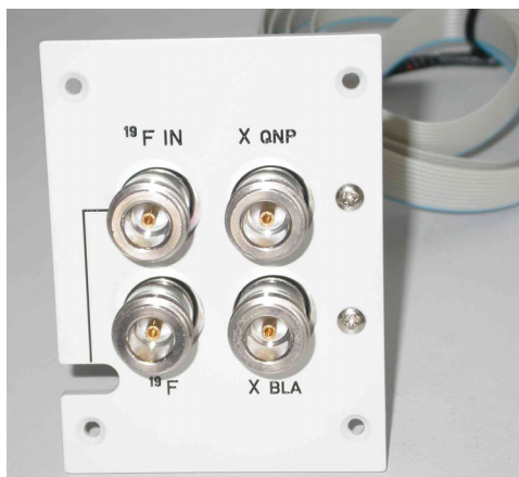
Figure 5.5. View of QNP Relay Accessory before installation
