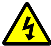
Figure 2.3. Electrical hazard symbol
