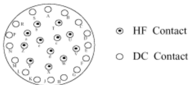
Figure 5.4. Back Panel Connector at AV Instruments (front view)
