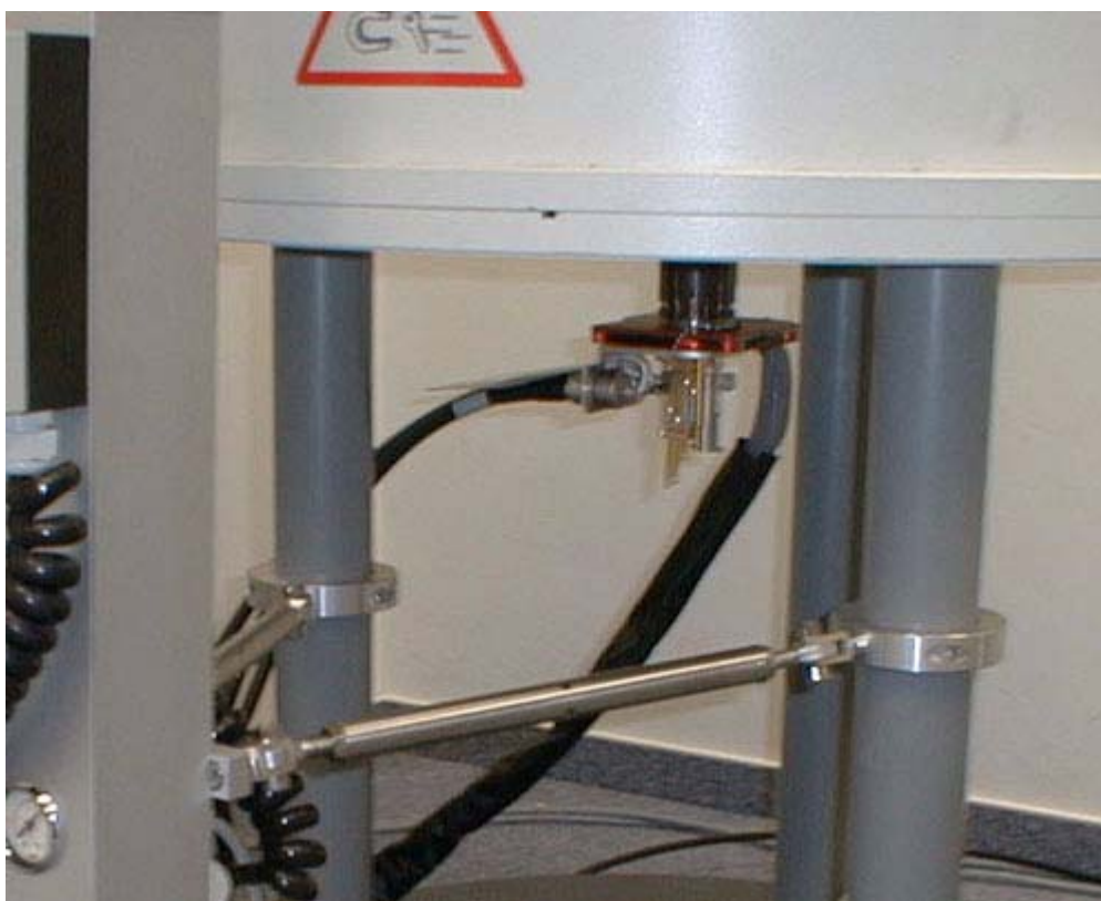
Figure 3.11. Adjustable Arm Assembly for Bottom of B-ACS
