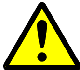
Figure 2.3. General hazard symbol
