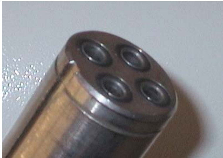
Figure 4.7. O-rings on the CryoCoupler
