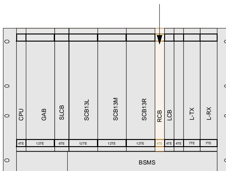
Figure 2.1. The location of the RCB in the BSMS Chassis
