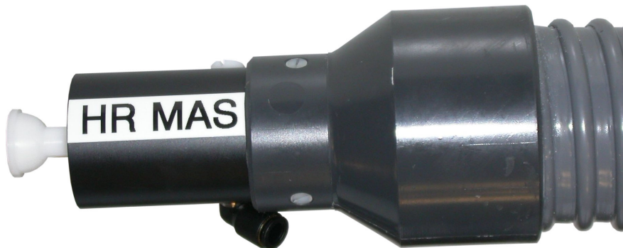
Figure 5.6. HR-MAS End Adapter mounted
