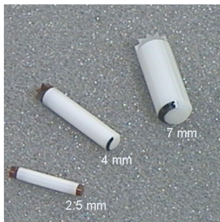
Figure 4.3. Markings at base of rotors
