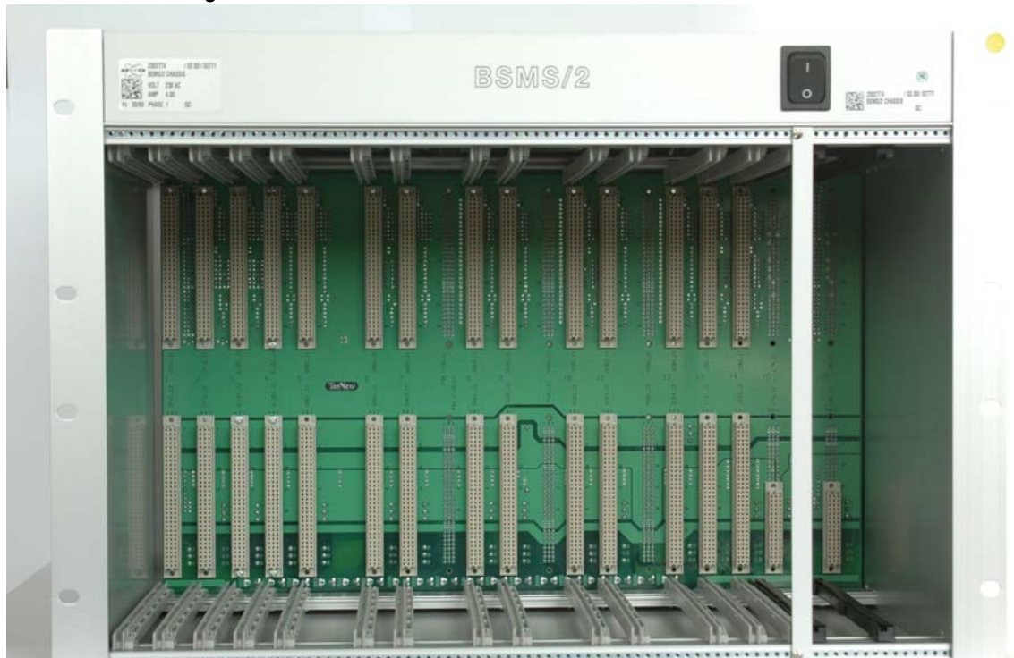
Figure 2.5. Front View of BSMS/2 Rack
