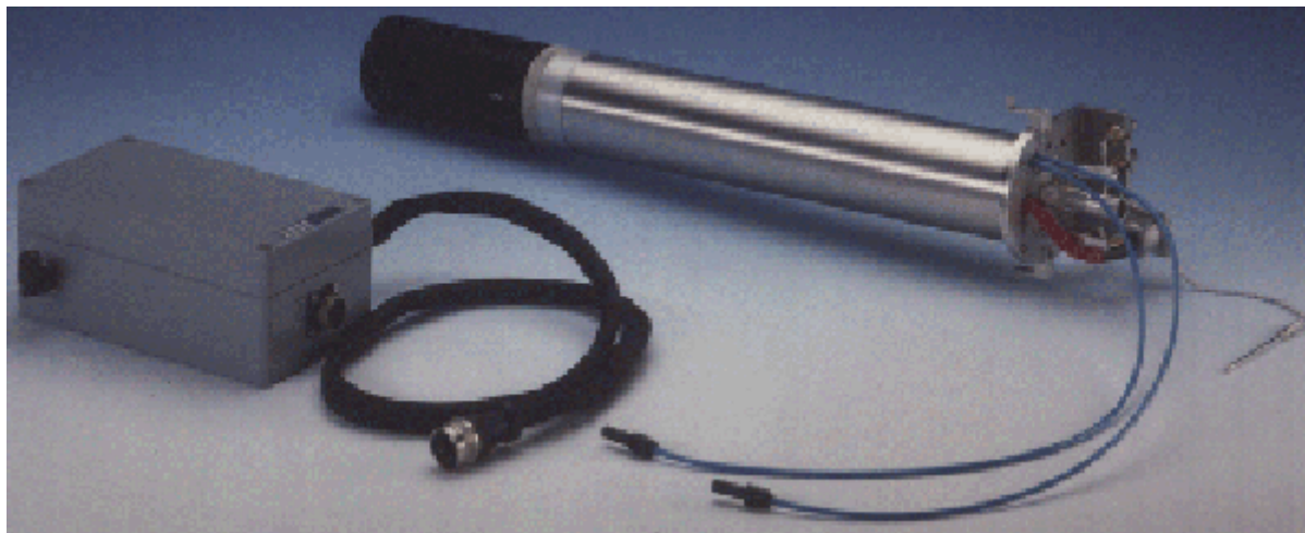
Figure B.1. Diff25 probehead, rf inserts and gradient security box
