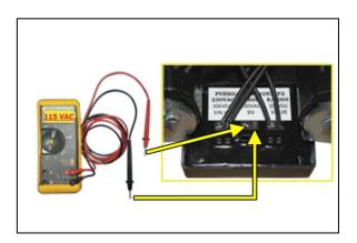
If the incoming voltage measures less than indicated above, it is recommended that steps be taken at your facility to increase the incoming power to the recommended levels.
