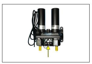
**8.3.3** Use a Voltmeter to measure the AC voltage across the "IN" terminals.
