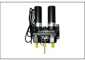
**8.4.3** Use a Voltmeter to measure the DC voltage across each set of "VALVE" terminals.
