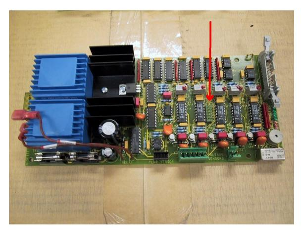
With the supervisor board positioned with the 2 blue transformers on the left (as shown above) the bank of jumpers, about an inch long, run vertically on a green base. The markings are as follows (top to bottom):
