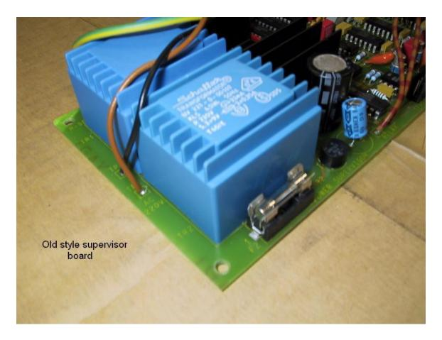
• Notice the two wires on the edge of the card next to the 2 blue transformers.
